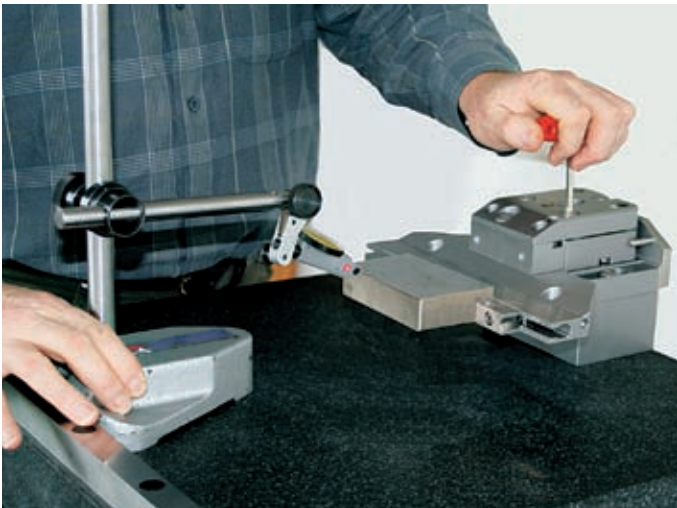
2. Accurately adjust the workpiece
