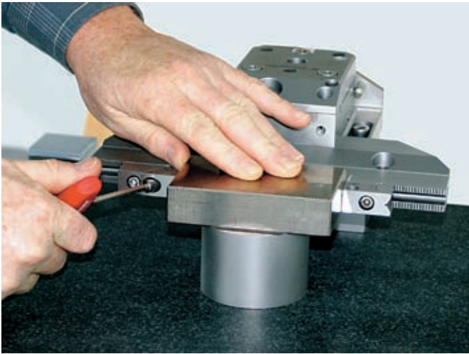
1. Clamp the workpiece in the holder
