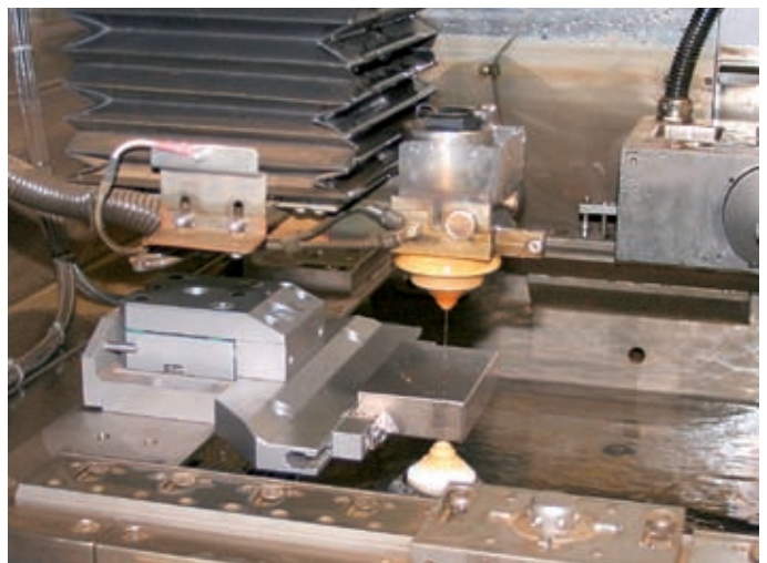
3. Erode the workpiece
